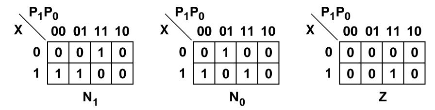
$$\begin{split} &N_1 = X\overline{P_1} + \overline{X}P_1P_0 \\ &N_0 = \overline{X}\overline{P_1}P_0 + XP_1P_0 + X\overline{P_1}\overline{P_0} = \overline{X}\overline{P_1}P_0 + X(\overline{P_1 \oplus P_0}) \\ &Z = XP_1P_0 \end{split}$$
